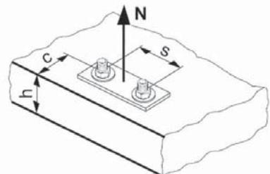
**Basic design tensile resistance****Design steel resistance  $N_{Rd,s}$**
