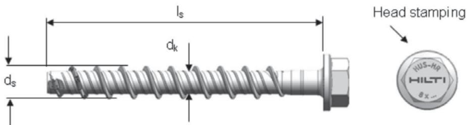
**Screw length and thickness of fixture for HUS-HR (hex head)**
