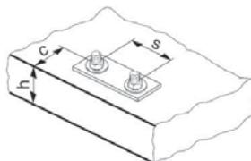
For spacing (edge distance) smaller than critical spacing (critical edge distance) the design loads have to be reduced (see system design resistance),
