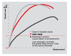
The pronounced undercut results in high rigidity and thus low anchor displacement. This makes the HDA a robust solution for fastening in cracked concrete.
