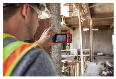
The PD-C laser range meter makes it possible to take photographs, measure distances and save these values directly in the photo.
